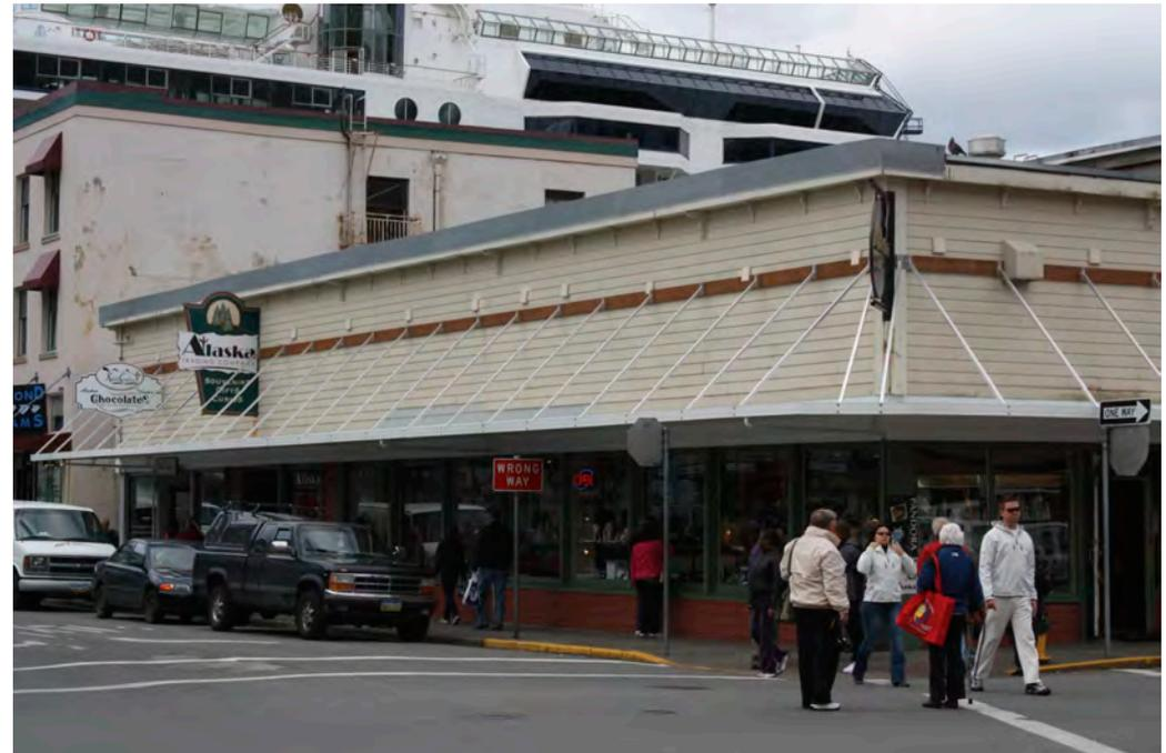
*When it was completed in 1912, the single-story, wood-frame Heckman Building 3 blended well with its immediate neighbors, the Revilla Hotel on Mission and Heckman's original wooden building on Main. Now, there is a marked contrast with the newer, concrete structures that flank it on both sides--a contrast accentuated by the loss of its transom windows and the gain of an out-of-period marquee.*
