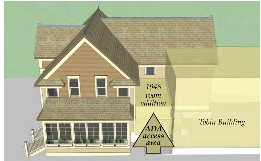
*This model illustrates a likely option for ADA access entering the building from the boardwalk on a ramp configuration that could enter the building at the north end of the restored entry porch.*
