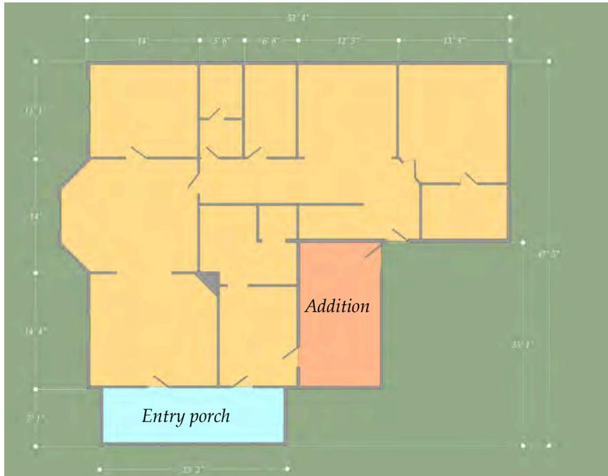
*The first and second floors total approximately 3,600 sf. A central staircase serves the second floor. There are two entries: one on the Mission Street elevation and one on the east elevation. The light blue in the first floor plan indicates the entry porch area; the red-orange indicates a room added to the building in 1946.*
